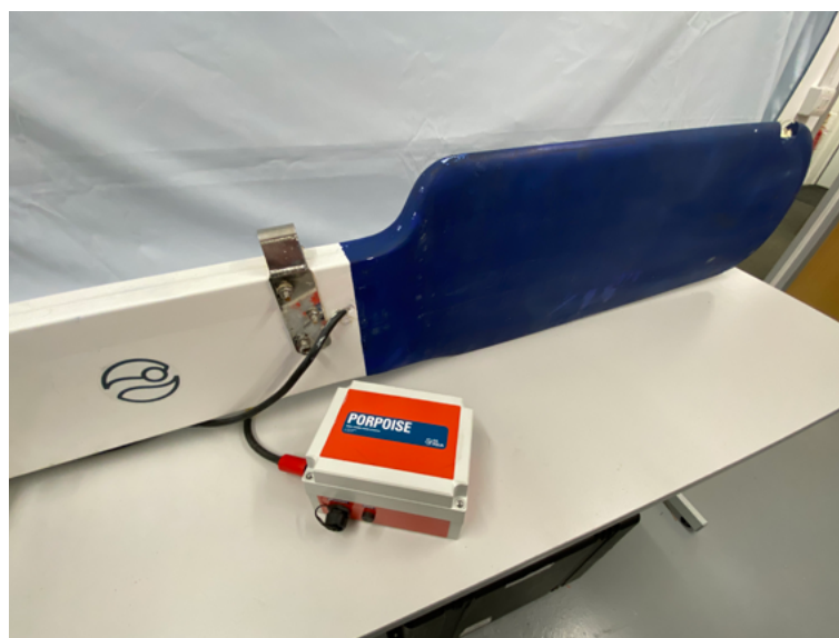
Image of the RS Aqua Porpoise hydrophone integrated with the rudder of a GB Row Challenge boat.
